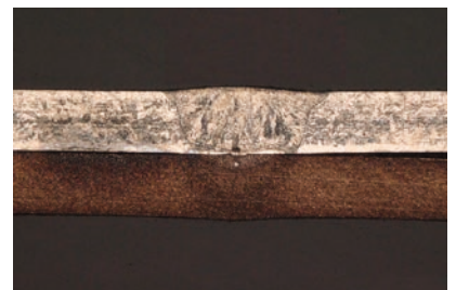
Fig. 4 This lap weld of 200-μm thick copper and stainless steel was produced by a 300-W blue laser working at 5 m/min. The joint displays reduced formation of intermetallics and minimal to no spatter and defects.
