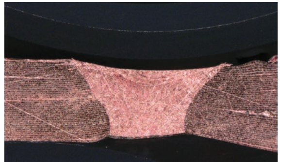
Fig. 5 Because blue laser welding is deterministic and stable, even very thin copper foils can be joined at high speed and with no defects.
