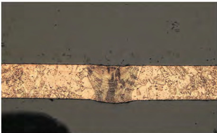
The same consistency leads to spatter-free blue laser keyhole welding. Magnification: \times 200 .
