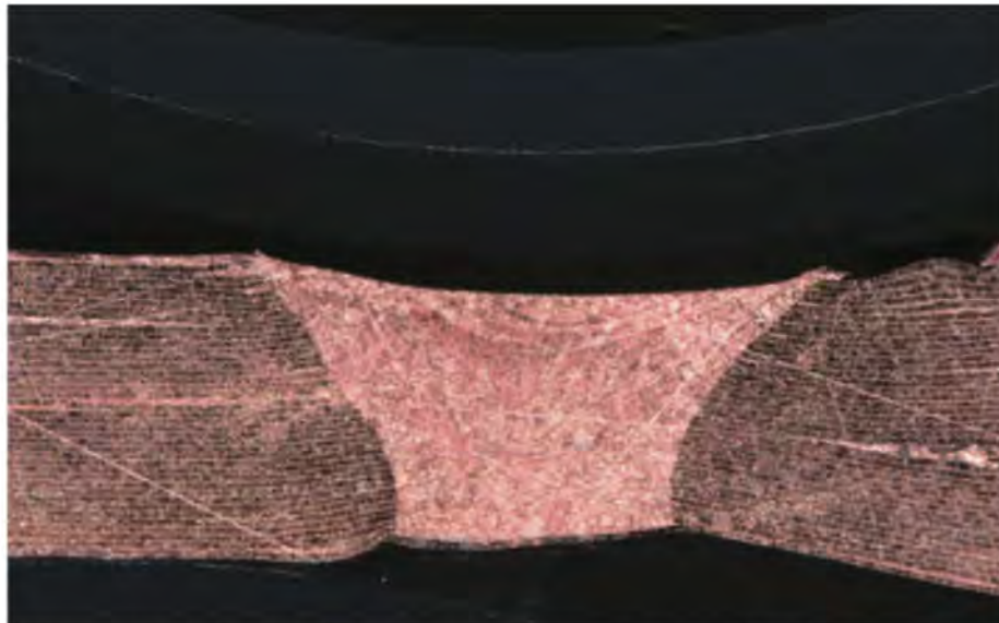
Blue laser welding of thin copper foils reliably produces defect-free welds, as shown in this image of the welding joint for 40 10- \mu\text{m} -thick foils.
